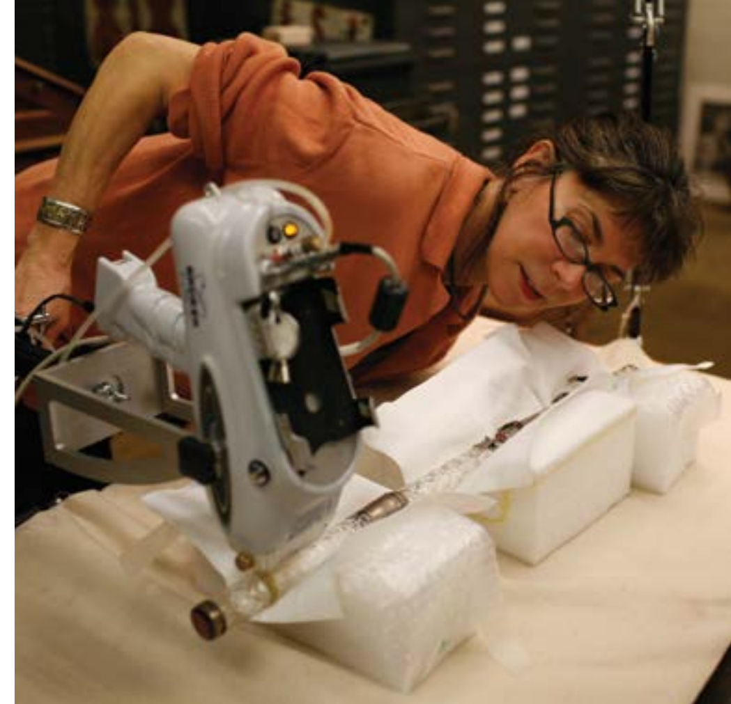
Lynn Brostoff of the Library’s Preservation Directorate performs an X-ray fluorescence analysis on a glass flute from the Dayton C. Miller flute collection in the Music Division. Photo by Abby Brack Lewis
